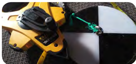
Figure 4: A secchi disk, which is used by Sherbrooke Lake volunteers to determine the clarity of the water.
